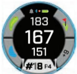
**Solid Blue Slope Ring** - *Indicates unit is calibrated and displaying Slope compensated distances.*
