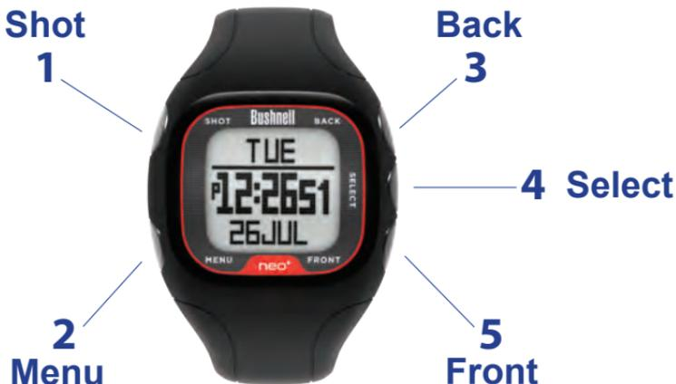
1. **SHOT Button:** Tracks shot distance in Play Golf mode. Controls backlight. Press & hold for night mode. Disable night mode with a single quick push. Press Select, Front, or Back to exit Shot Distance.
